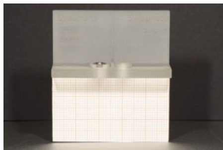
Fig. 1. Study set-up. A standard metal sleeve is incorporated into the left control site; no metal sleeve is present in the printed test site at the right. The same set-up was used for Test 1/Control 1 and Test 2/Control 2, with the respective sleeves corresponding to the surgical system.
