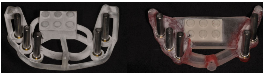
Figure 2 Titanium pins were inserted into the sleeves, allowing to determine the expected implant deviations if used for surgery.
